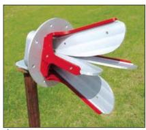
Fig. 14 The final configuration of the proposed antenna.
