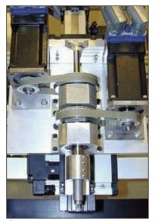
Fig. 4 Coaxial screw/nut driver to handle standard tuning screws and lock nuts.
