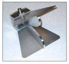
immunity and emissions testing horn. It has also been tested for compact range illumination, showing a good performance in the low end of the frequency range and a small reduction in the diameter of the quiet zone (QZ) at the upper end. This horn was designed using MW Studio, a commercial package based on the finite integration time domain technique.
