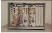
Fig. 7 A standard C-size VXI-based SI VNA/SA.
